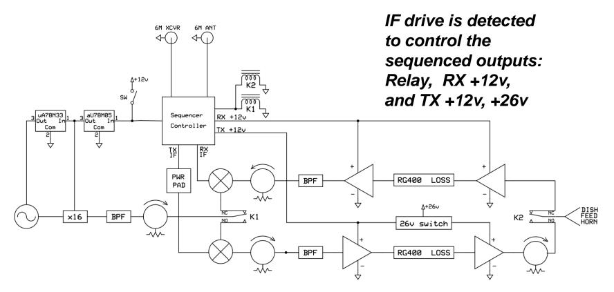
LNA and PA are located with a SMA coaxial relay at the dish horn-feed
